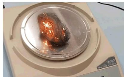
Step 4 When the reaction is complete read the mass from the scale.
