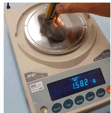
Step 3 Allow the wool to slowly burn. Reignite with the battery if necessary.
