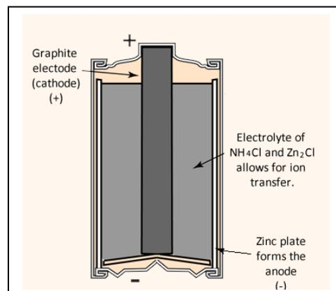
1) Although the overall cell reaction for this battery is complex we can break it down into two major reactions.
