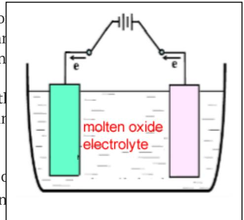
Electrolysis produces iron a different way. The iron ore (Fe<sub>2</sub>O<sub>3</sub>) is dissolved in a solvent of silicon dioxide and calcium oxide at 1600°C and an electric current passed through it. Negatively-charged oxygen ions migrate to one electrode producing oxygen gas that is allowed to bubble off. Positively-charged iron ions migrate to the other electrode where they are reduced to elemental iron which collects in a pool at the bottom of the cell and is siphoned off.
