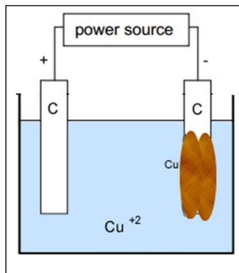
b) The same electrolytic cell was used by a student to produce copper metal. A current of 25.0 Amps was passed through the cell for 12 hours. What mass of copper was deposited?
