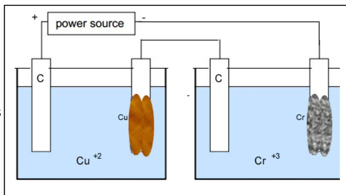
Example 6 A charge of 0.250 Faraday was passed through an electrolytic cell with 0.100M solution of  $\text{CuSO}_4$ , as shown on the right.
