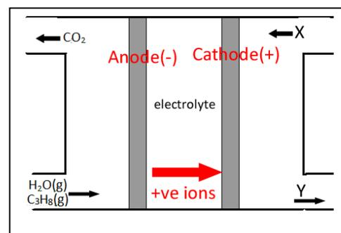
2) Molten carbonate fuel cells (MCFCs) use a molten carbonate salt suspended in a porous ceramic matrix as the electrolyte. Salts commonly used include lithium carbonate, potassium carbonate and sodium carbonate. They operate at high temperature, around 650°C and the benefit of this is that the rate of reaction at both electrodes is significantly increased. This eliminates the use of expensive catalysts to improve the rate of reaction.
