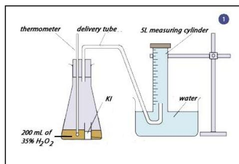
1. Set up the apparatus as shown on the diagram
