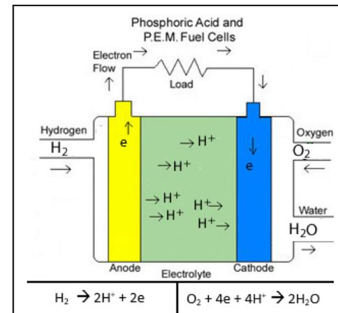
Writing half reactions for fuel cells. Writing half reactions for an alkaline or acidic fuel cell is identical to writing half equations for an alkaline or acidic galvanic cell. Keep in mind that the fuel always goes at the anode (-) of a fuel cell.
