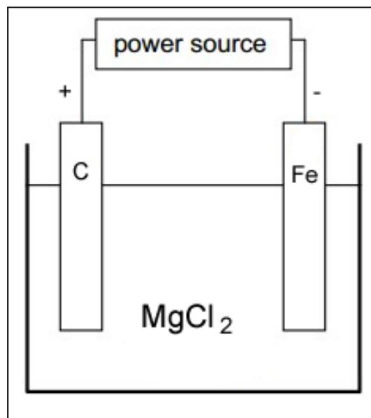
d) The polarity of the electrodes were accidentally changed by the student, as shown on the right
