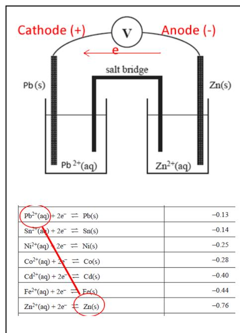
Consider the two galvanic cells shown on the right operating at standard conditions.
