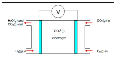
$\text{Na}_2\text{CO}_3$  as the electrolyte. Hydrogen gas is passed over one electrode and a combination of oxygen gas and carbon dioxide gas is passed over the other electrode, as shown in the diagram below. The net overall reaction is  $\text{H}_2(\text{g}) + \text{O}_2(\text{g}) \rightarrow \text{H}_2\text{O}(\text{g})$ . There is no net gain or loss of the electrolyte.
