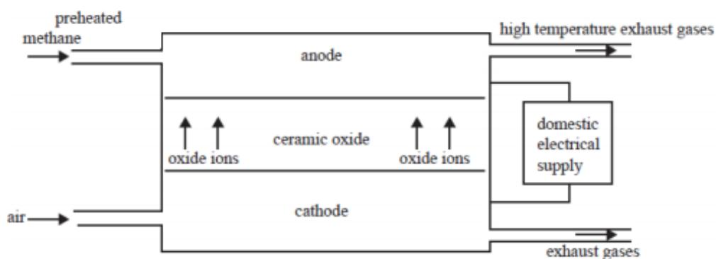
They operate at temperatures in excess of  $500^{\circ}\text{C}$ .
