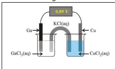
The cell potential was measured at 0.89 V, with the copper electrode gaining mass when the cell was discharging.
