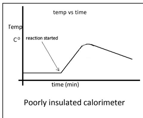
To find the final temperature of the solution in the calorimeter we extrapolate backward the line of decreasing temperature, as shown on the right, in red. The point where the extrapolated line and the starting temperature intersect is the final temperature.
