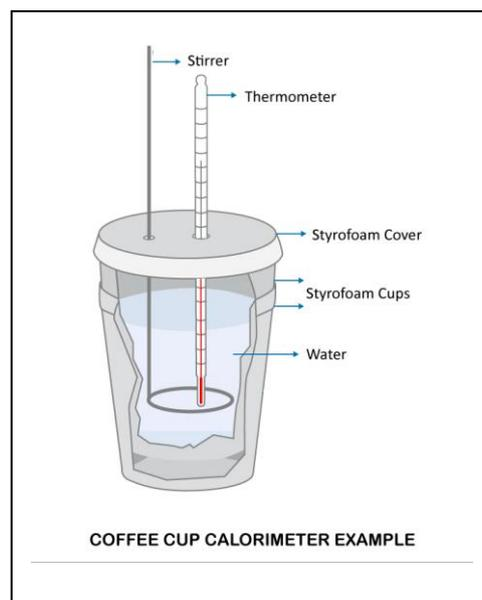
In order to accurately determine the energy lost or absorbed by the reaction we must first calibrate the calorimeter. This is done by delivering a known amount of energy, most often done by passing a known electric current at a given voltage for a period of time measured in seconds. The change in temperature of water is then measured and the calibration factor ( $C_f$ ) determined.
