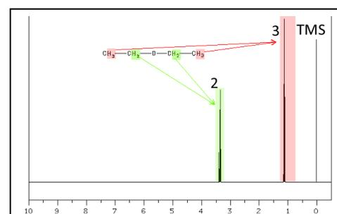
**Ppm**—The horizontal scale of an HNMR spectrum is shown as (**ppm**). It is called the chemical shift and is measured in **parts per million - ppm**. It increases as we go from right to left and a peak at a chemical shift of, say, 3.0 means that the hydrogen atoms which caused that peak need a magnetic field three millionths less than the magnetic field needed to produce the TMS signal.
