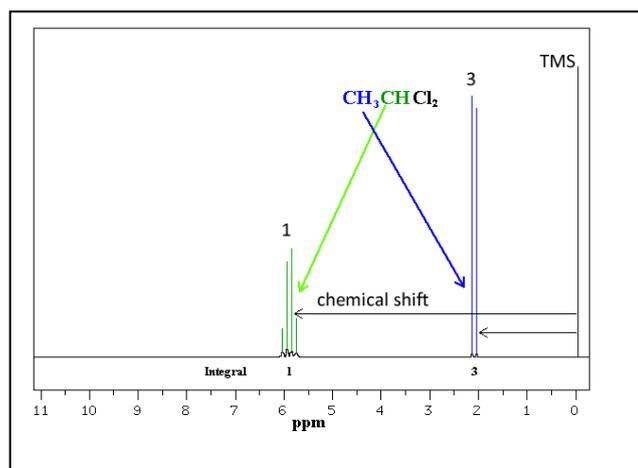
**Shielding**— Electrons surrounding hydrogen nuclei (protons) shield the nucleus from the applied magnetic field, the greater the electron density the greater the shielding. Hydrogen nuclei which are close to electronegative atoms, such as oxygen or chlorine, experience much lower shielding than hydrogen nuclei which are further away from an electronegative atom. Lesser shielding causes the signal from a hydrogen nucleus to move further over to the left on the spectrum, greater chemical shift.
