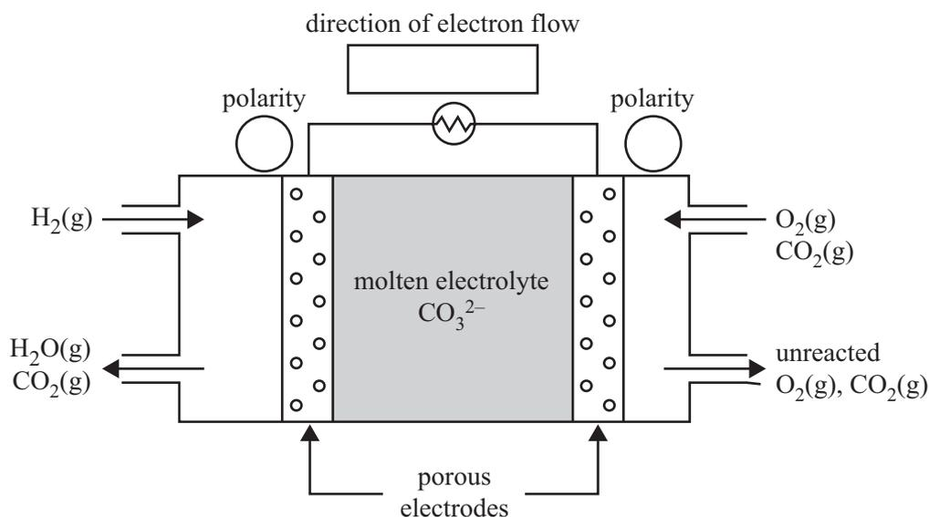
At one electrode of the MCFC, carbon dioxide,  $\text{CO}_2$ , gas reacts with oxygen,  $\text{O}_2$ , gas to form carbonate ions. At the other electrode, hydrogen,  $\text{H}_2$ , gas reacts with molten carbonate ions to form steam and  $\text{CO}_2$  gas.
