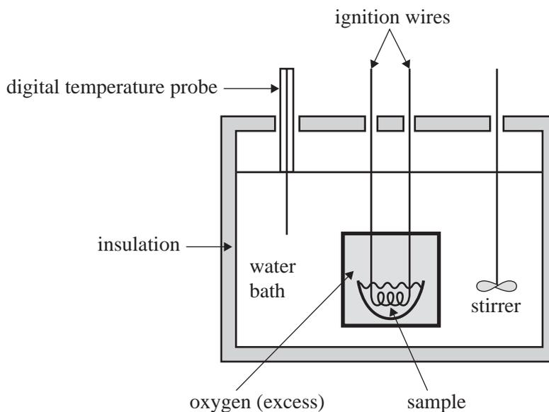
The calibration factor for the bomb calorimeter is initially determined by burning a known amount of naphthalene,  $C_{10}H_8$ .
