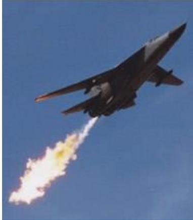
The forces acting on it include drag, lift, gravity and thrust. Obviously the plane is acted on by unbalanced forces. Since the plane is **accelerating**, the force of lift is greater than the force of gravity and thrust is greater than drag.
